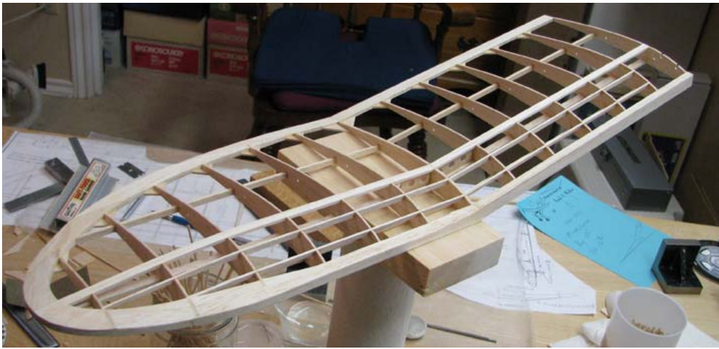
The new wing panel was integrated into the salvaged wing structure.
