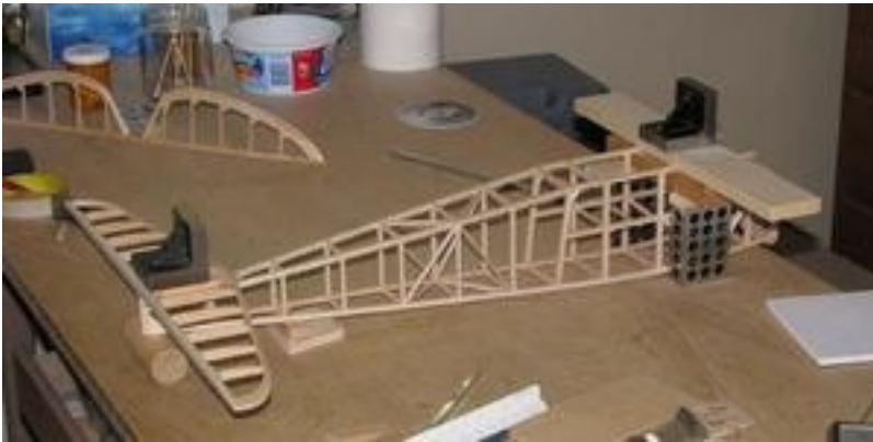
Jigging for Stab Mounting Platform
