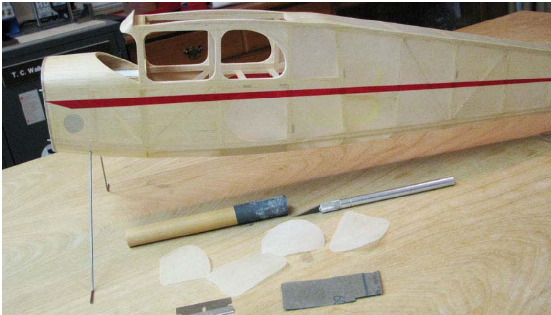
The windshield and side windows of 0.005" clear Dura-Lar were installed.
