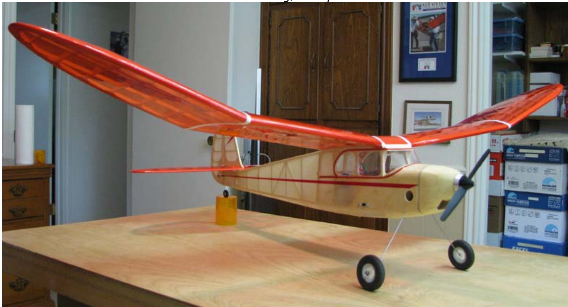
The Cloudster's balance point is at 48.7% as per the Jim Adam's plan and the total weight is 16.05 ounces.....Tandy
