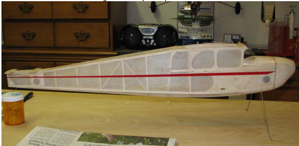
The fuselage and cowl were given one thin air brushed coat of clear satin Klass Kote.
